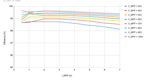
Efficiency of Elmar Solar's Best MPPT (2021) V\_OUT = 120V
